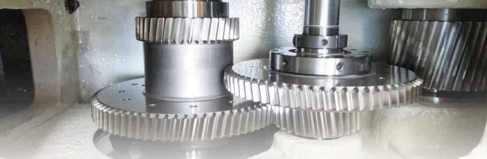
FANUC α15/8000 15KW / 18.5KW Drive type: Gear (#50) Max. spindle speed: 6000rpm
