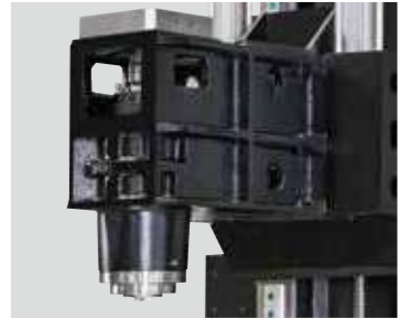
Direct drive spindle and loge nose cast iron one piece structure.
