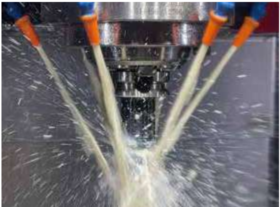
Coolant Jets Around Spindle
